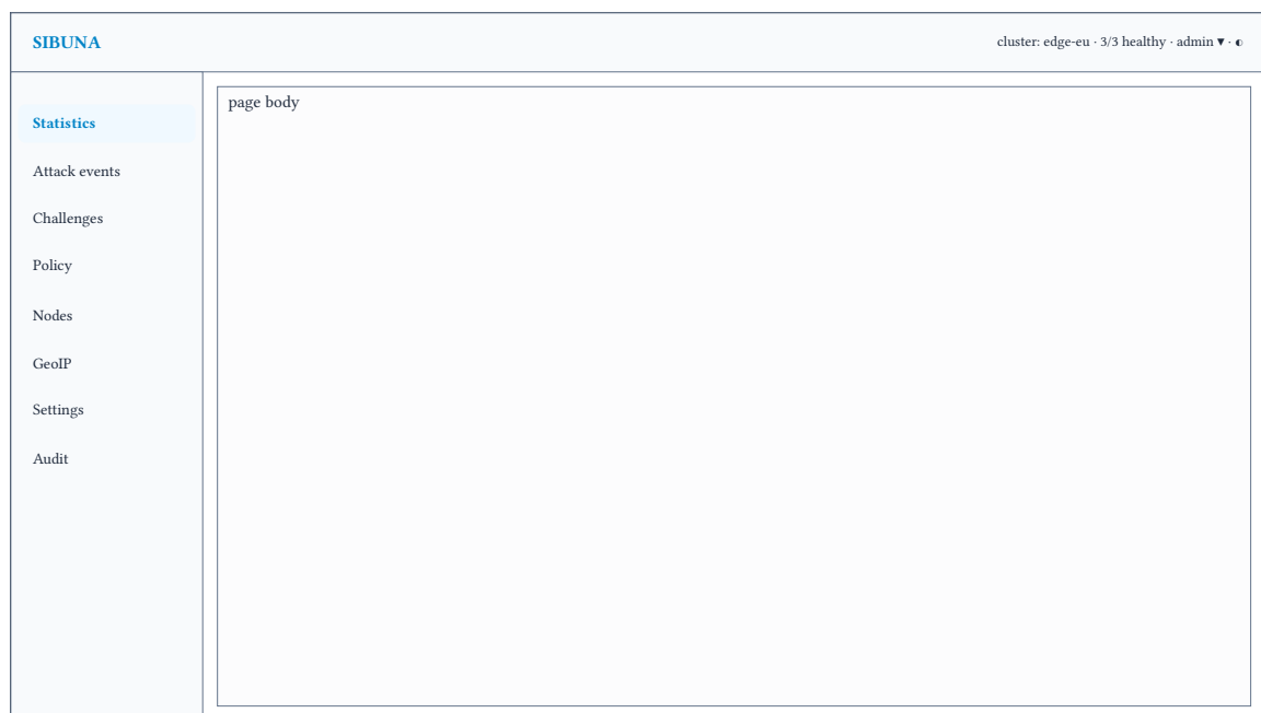
Figure 23: The shell: top bar with cluster status and the account menu, a fixed sidebar of the eight pages, and the page body. Below 1,024 px navigation becomes a labelled menu drawer.
