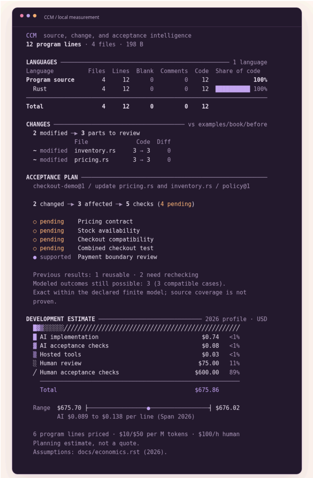
Fig. 3 One change report connects file differences, affected parts, evidence, and resource assumptions.
